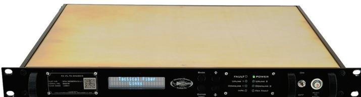
Ka-band fiber optic interfacility link
